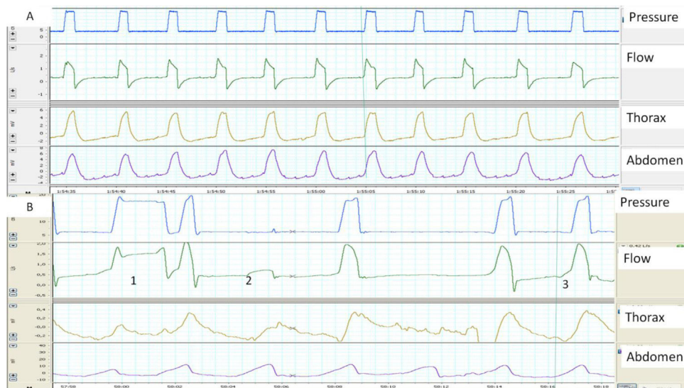
Fig. 1. (A and B) Examples of normal and pathological patient-ventilator synchrony, determined with the help of thoracoabdominal belts. (A) The image shows perfect synchrony between the patient's thoracoabdominal movements and the ventilator cycles (continuous line). (B) The image of cycle 1 shows a long cycle, presumably due to leakage (the patient has finished exhaling while the ventilator continues in inspiration) and cycle 2 displays an ineffective respiratory effort (movement of belts without pressurization). Finally, in cycle 3, the beginning of the ventilator cycle is delayed with respect to the start of the movement of the belts (trigger delay, more apparent in the abdominal belt).
