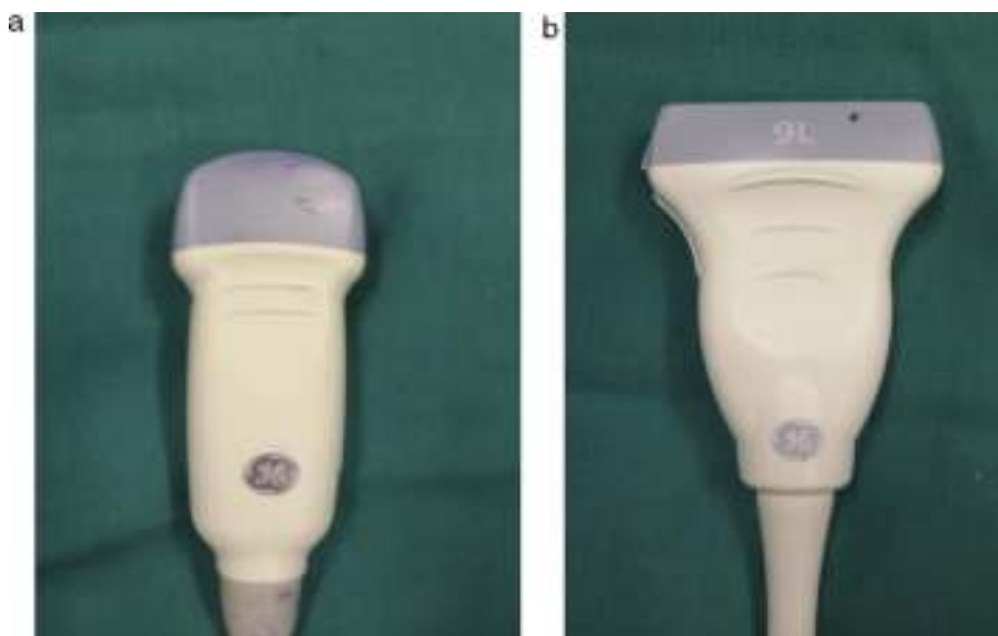
Fig. 1. Photo of the convex (a) and linear (b) transducers.
