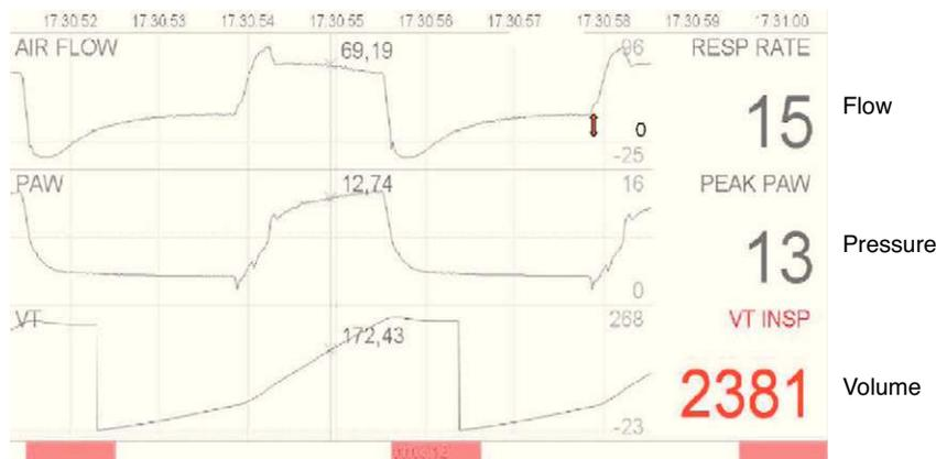
**Fig. 9.** Method for calculating leaks. The system detects the transition between the expiratory and inspiratory flow slopes. The flow that at that time is circulating through the pneumotachograph (double arrow) is considered by the system as a leak flow.
