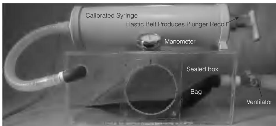
**Figure 1.** Bag-in-Box Lung Simulator System. The 2-L bag is connected to the ventilator and the 8-L box is connected to a 3-L calibrated syringe with an elastic recoil to depress the plunger.
