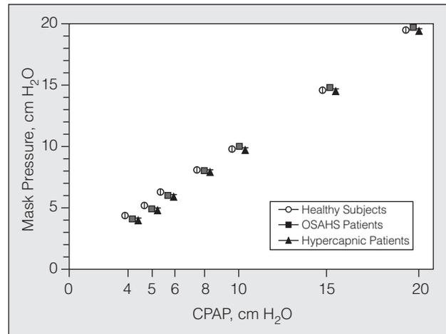
Figure 2. Pressures achieved in the prototype mask during application of CPAP in the 3 study groups. OSAHS indicates obstructive sleep apnea-hypopnea syndrome.
