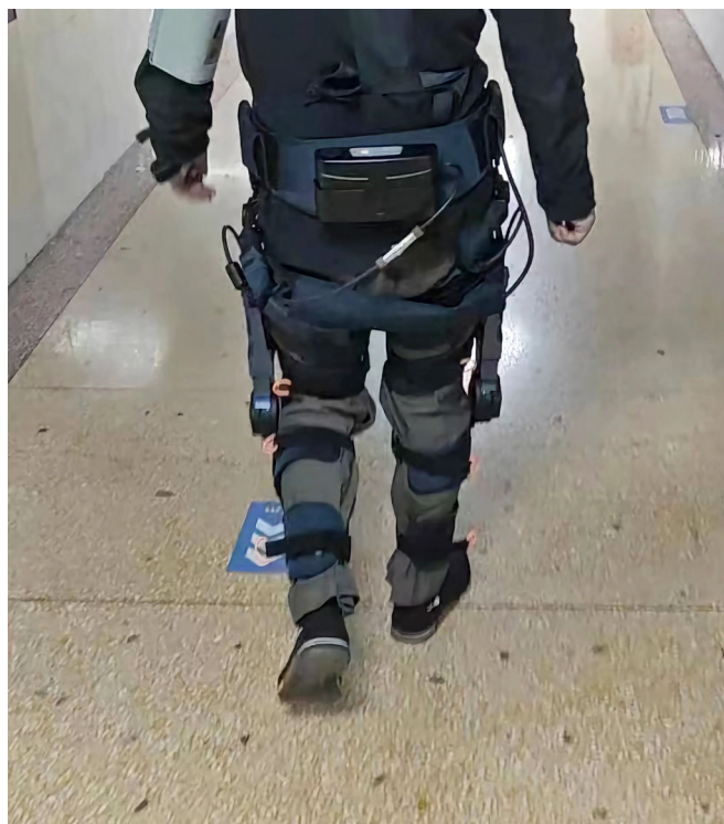
Fig. 1. The patient with chronic obstructive pulmonary disease (COPD) wore the exoskeleton during practicing 6-minute walk test (6MWT).
