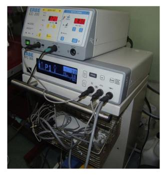
Figure 1. ICC 200 electrosurgical generator workstation, ERBE, Germany.
