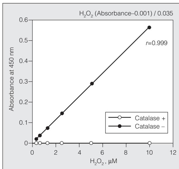
Figure 1. Calibration curve prepared using a standard solution of hydrogen peroxide (H<sub>2</sub>O<sub>2</sub>). Black circles indicate untreated solution and white circles solutions pretreated with catalase.
