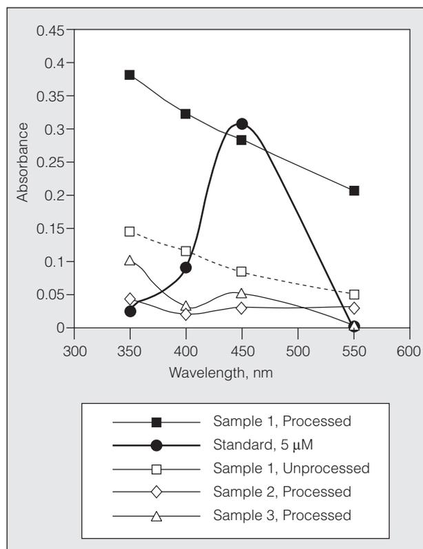
Figure 3. Absorption spectrum following processing of a 5 µM standard solution of hydrogen peroxide and 3 patient samples. The spontaneous absorption spectrum of an unprocessed sample is also shown. Only the standard solution displays an absorption peak at 450 nm.
